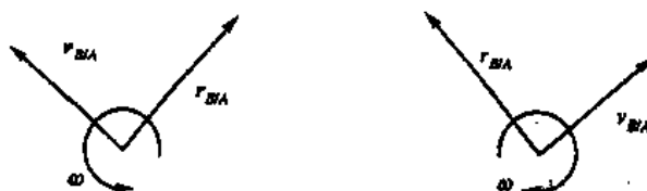
Fig.6.5.4 The Direction Relationship Among the Vectors v_{B/A} , \omega , and r_{B/A} for Planar Motion
